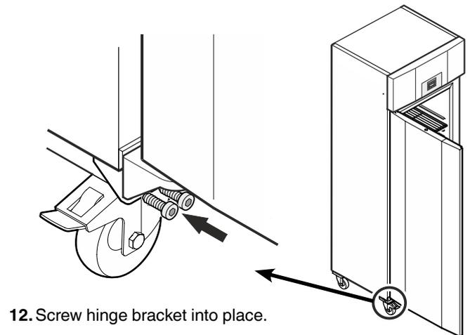
12. Screw hinge bracket into place.
