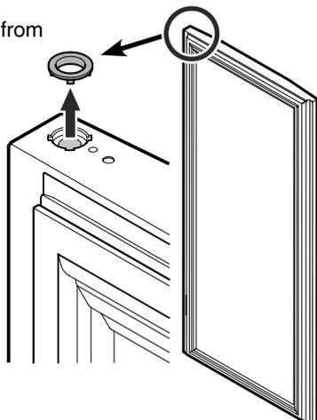
4. Remove the hinge components from the hinge bracket.
