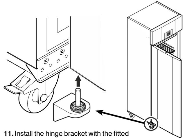
11. Install the hinge bracket with the fitted hinge components in the lower door mounting.
