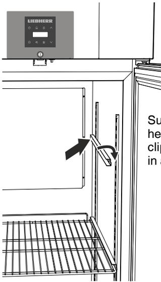
Suspend the rails at the desired height, by inserting into the rear clip-in strip first and then clipping in at the front.
