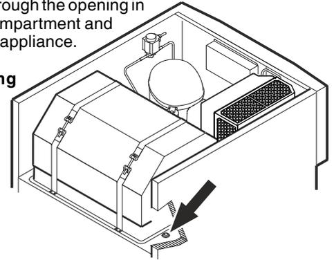
2. Undo the screw on the underside of the front panel. Tilt the front panel upwards.
