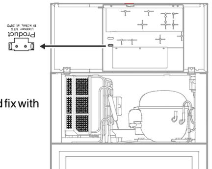
4. Close the front panel and fix with the screw.
